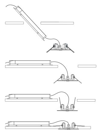
4. When the mains supply to the fitting is energised the green indicator LED located on the lamp head should illuminate. As this product is non-maintained, the emergency LED will not illuminate unless there is a power failure, or the test button located on the lamp head is pressed. If the charging indicator LED does not illuminate, then check that the battery and lamp head cables are properly plugged into the main control unit and refer to the troubleshooting guide at the end of this document.
